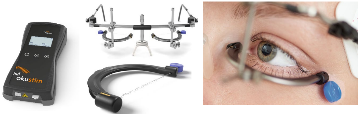
Fig. 2: OkuStim System. Left: OkuStim device. Centre: OkuSpex frame (top) holder for OkuEI electrodes (bottom). Right: During stimulation, the electrode thread is in contact with the conjunctiva and cornea below the pupil.
